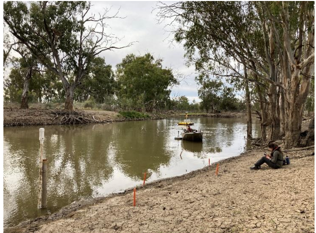
Photo 2: DEW staff undertaking gauging in the Chowilla anabranch creeks to ensure good flowing conditions for Murray Cod during the weir pool lowering at Lock 6.
